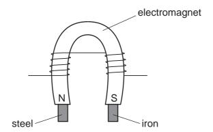
The current to the electromagnet is switched off.
