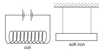
The current is then reversed by reversing the battery connections.
